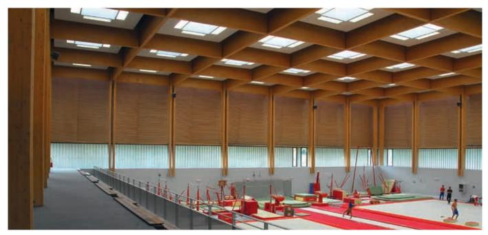
The 12,000 m<sup>2</sup> of the building have been fitted with Versatile Reverse radiant ceiling panels which build a frame around the lighting. A total of 1836 m<sup>2</sup> blends perfectly into the idiosyncratic architecture.
