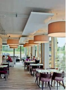
The climate in all of the office areas, including the cafeteria, is controlled with Versatile Carboline. The lightweight panels with natural graphite ensure particularly rapid, even and efficient temperature distribution.
