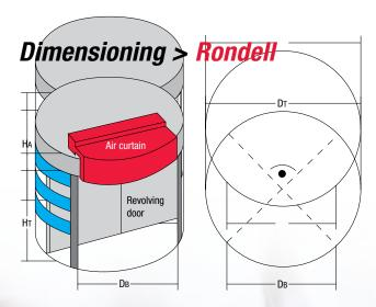
For dimensioning the revolving door unit, the following main measurements are required:
