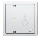
The Zehnder 12V 0-10V remote CO2 sensor and combined three position switch is designed to enable the user to manually select the desired ventilation systems flow rate based on the visual air quality indicator, or automatically adjust the unit relevant to the CO2 level.
