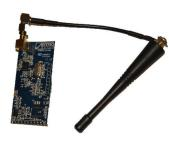
The Zehnder RF-PCB enables the CCRFZ (655 000 755) controller to be used with the ventilation system without the need for the ComfoSense C67.
