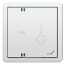
The Zehnder CO2 sensor C67 is a remote CO2 sensor and combined three position switch designed to enable the user to manually select the desired ventilation systems flow rate based on the visual air quality indicator, or automatically adjust the unit relevant to the CO2 level.
