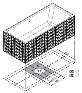
Adequate position to connect the drainage
