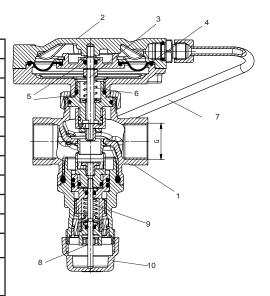
The use of ethylene and propylene glycol in a mixture ratio of 25 - 50% by volume [%] is permitted. Ammonia contained in hemp damages brass valve housings. EPDM seals are swollen by mineral oils or lubricants containing mineral oil and thus lead to failure of the EPDM seals. For frost and corrosion protection agents based on ethylene and propylene glycol can be found in the manufacturer's documentation.
