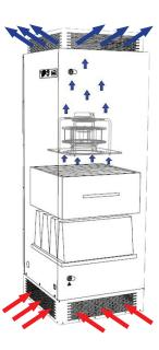
ALARM FILTER He (TD): ON IN POS.5. If The intervencement Constant air flow regulation guarantees the same level of safety against virus contamination regardless of the clogging of the filter.
