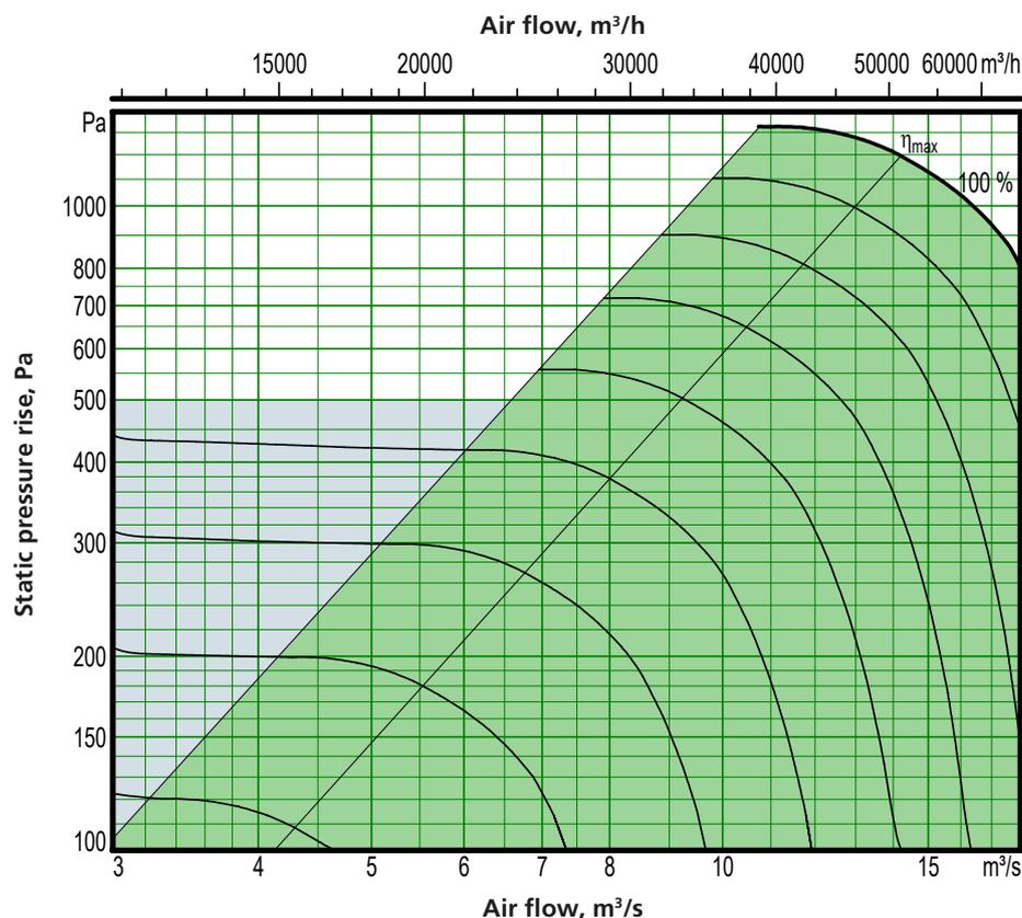
Motor shaft power: 3 x 10 kW (capacity variant 2)
