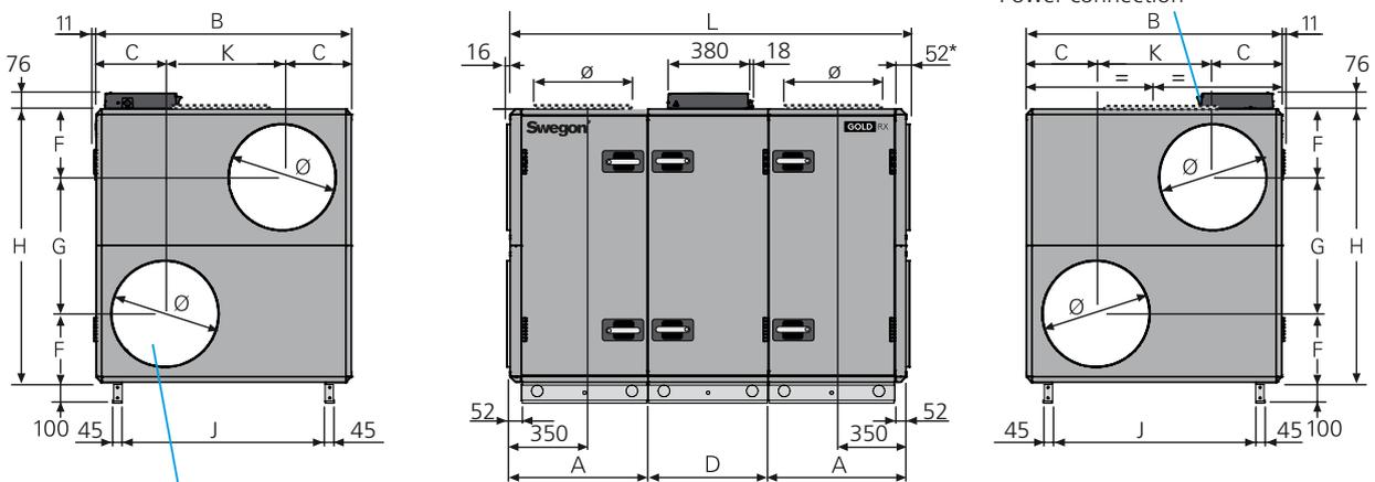
The illustration shows the connections for supply air fan, right-hand/lower level and left-hand/upper level. For supply air fan, right-hand/upper level and left-hand/lower level, the connections are mirror-inverted. \* The air handling unit is supplied without end connection panel if a duct accessory housed in an insulated casing will be connected. The AHU can also be supplied with full face end connection panel (accessory).
