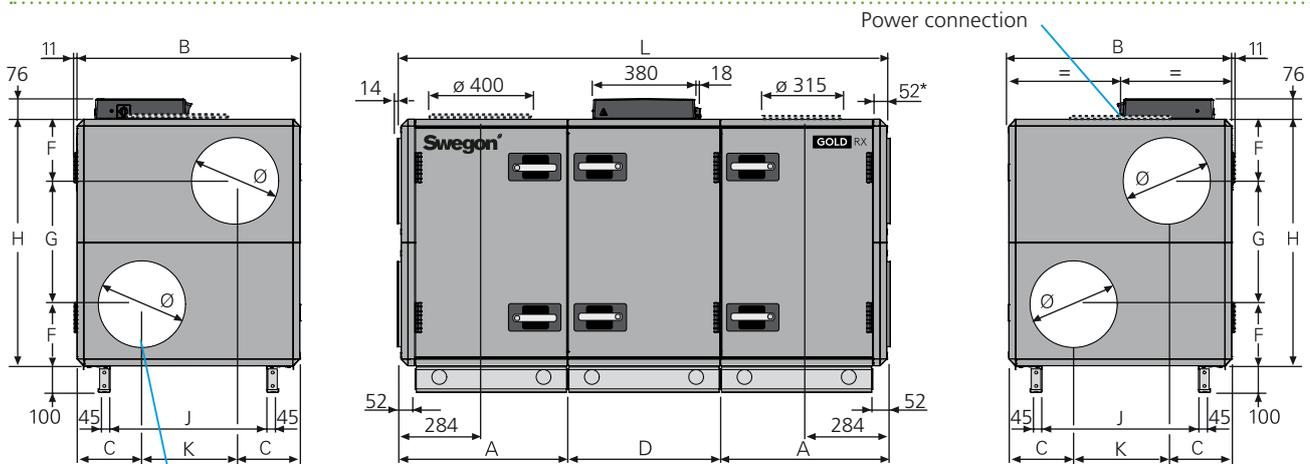
The illustration shows the connections for supply air fan, right-hand/lower level and left-hand/upper level. For supply air fan, right-hand/upper level and left-hand/lower level, the connections are mirror-inverted.
