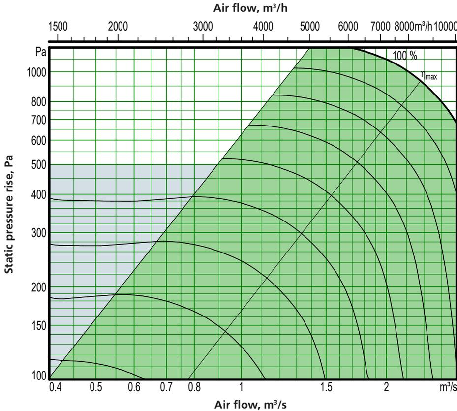
Motor shaft power: 3.4 kW (capacity variant 2)
