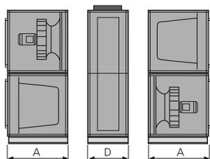
The unit can be divided into three sections at the building site. **Dimensions:** See A and D in the table above. **Weight:** A = 146-189 kg, D = 158-176 kg.
