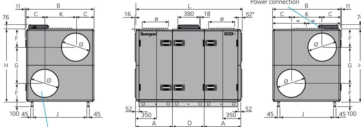
The illustration shows the connections for supply air fan, right-hand/lower level and left-hand/upper level.
