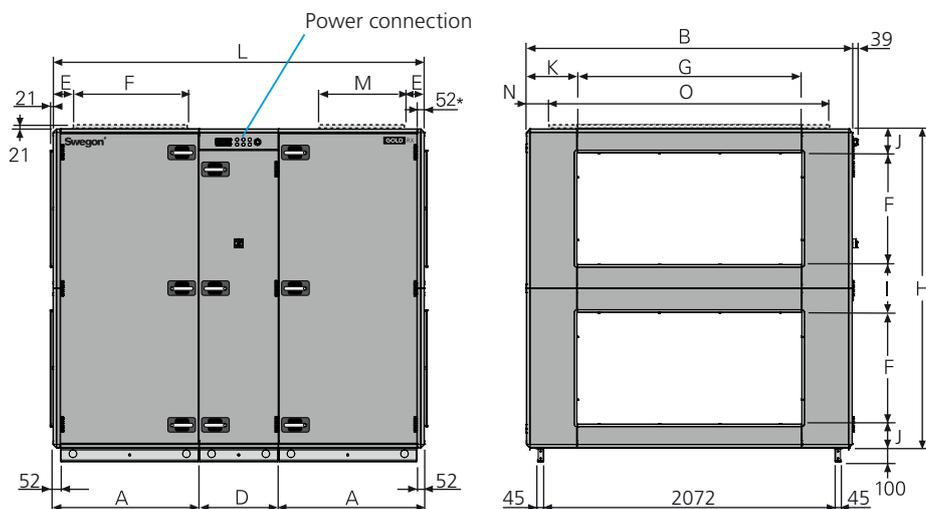
\* The air handling unit is supplied without end connection panel if a duct accessory housed in an insulated casing will be connected. The AHU can also be supplied with full face end connection panel (accessory).
