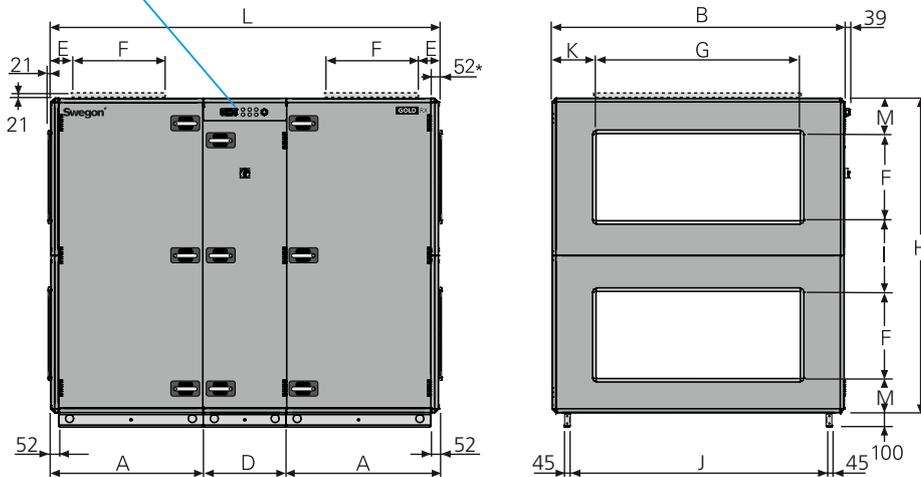
\* The air handling unit is supplied without end connection panel if a duct accessory housed in an insulated casing will be connected. The AHU can also be supplied with full face end connection panel (accessory).
