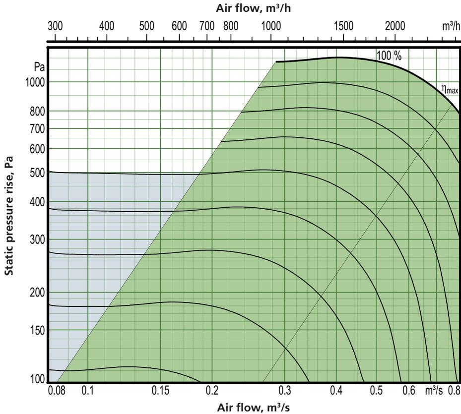
Motor shaft power: 1.15 kW (capacity variant 2)
