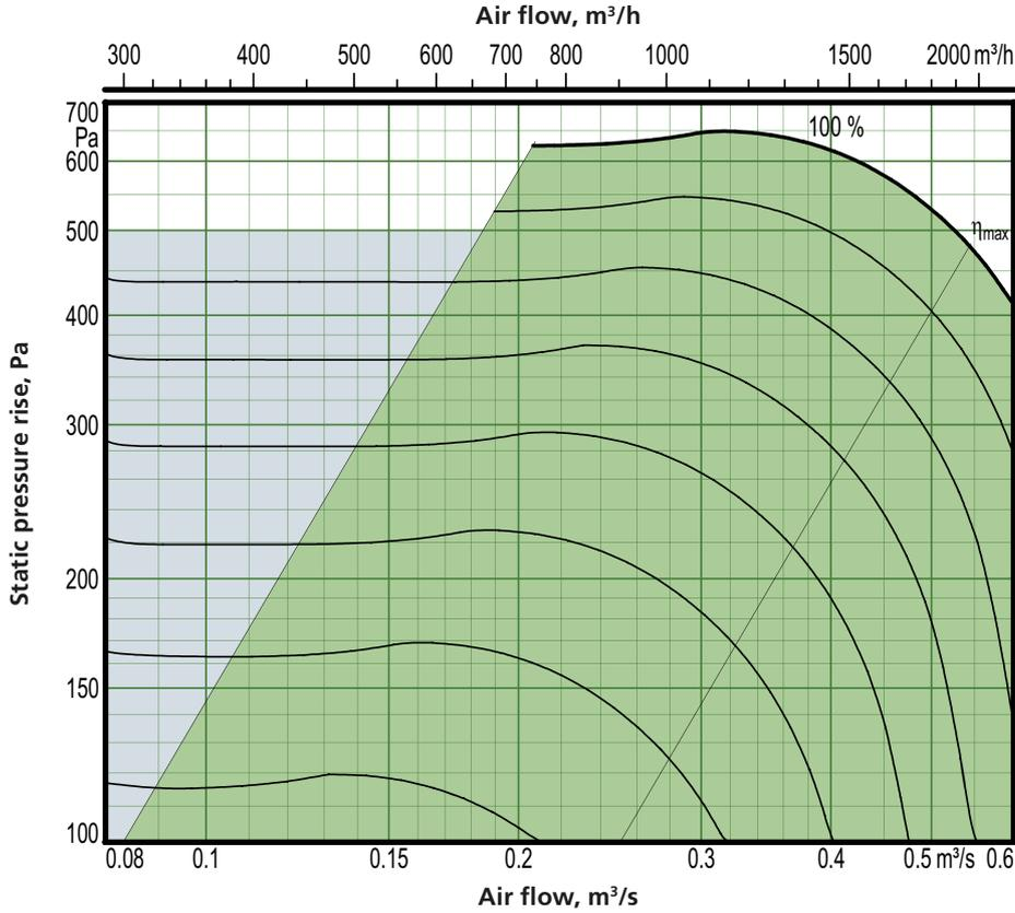
Motor shaft power: 1.15 kW (0.41 kW)
