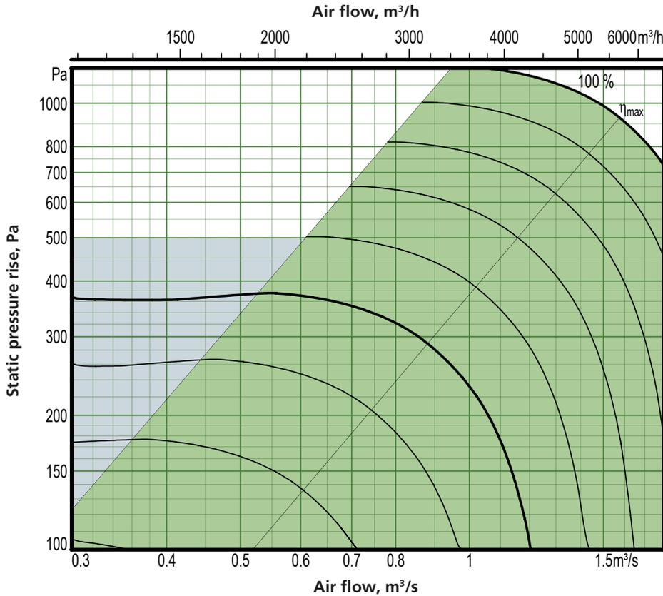
Motor shaft power: 2.4 kW (capacity variant 2)
