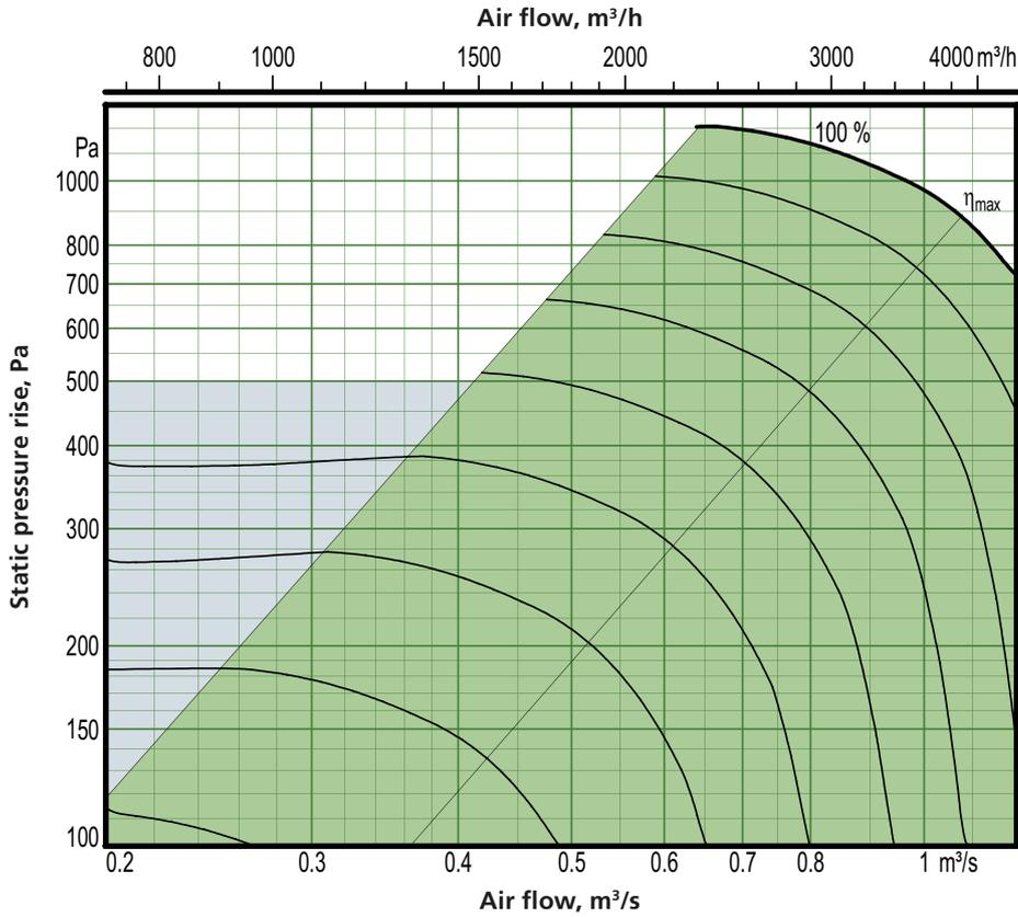
Motor shaft power: 1.6 kW (capacity variant 2)
