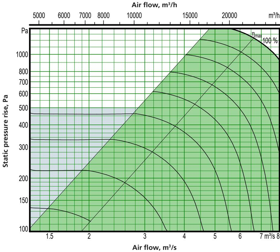
Motor shaft power: 2 x 6.5 kW (capacity variant 2)
