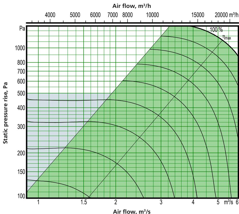
Motor shaft power: 10 kW (capacity variant 2)
