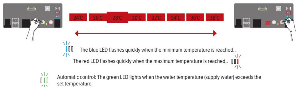
3. Exit setup mode: press and hold the [+] button until the red LED flashes 5x and release. Wait 15 seconds – the new setting will be saved automatically.
