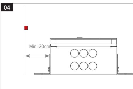
Place the device in the correct position..
